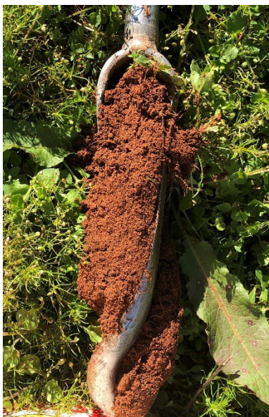
Collecting soil with an auger.
