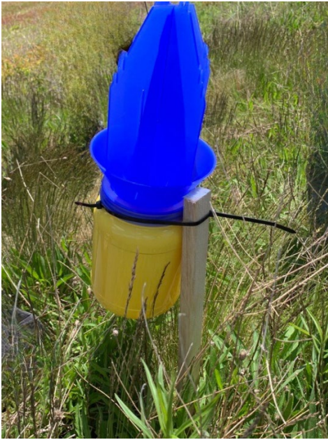
Blue vane traps are used to monitor bee population in living lab shelterbelt sites.
