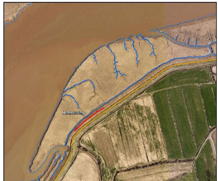
Figure 8: Location and extent of contemporary armouring of dyke. Although the location of the armouring is symbolized on the dyke segment, it represents armouring of the foreshore marsh.
