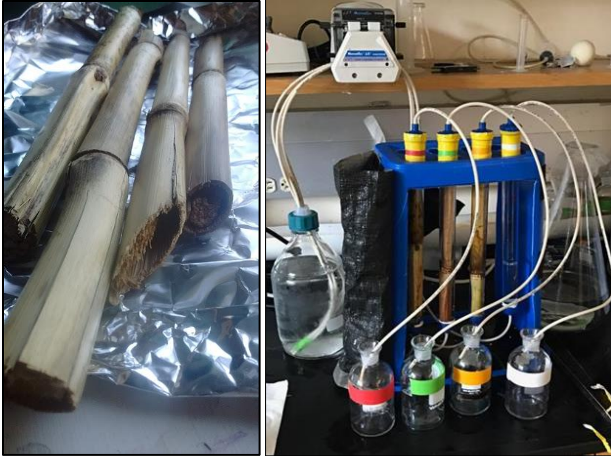
Figure 4. Left: Dried whole corn stocks, Right: Column denitrification test apparatus with 4 columns in operation (three with corn stalk, one blank)
