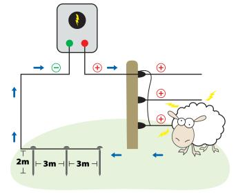
Fig. 3 The circuit is complete when the animal touches the wire. This figure shows the correct ground rod placement.
