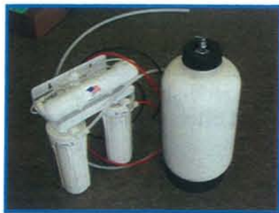
Reverse Osmosis System Used to Remove High Levels of Arsenic
